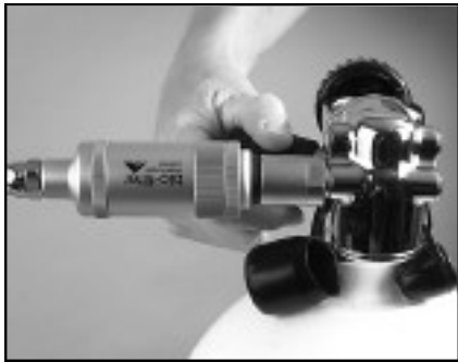
Step 13: Attach the regulator to a scuba cylinder valve and slowly turn the air on.
