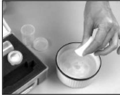
Step 8: Soak the Moisturizer Pad in distilled water. Squeeze out the excess water once it is completely soaked through.
