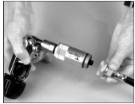
Step 6: Unscrew the Moisturizer Cap from the Bio-Filter.
