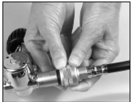
Step 3: Screw together the Moisturizer Cap and the First Stage Body Joint. Be sure to pressurize and check for leaks before diving.
