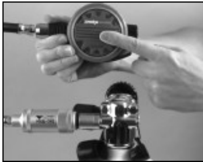
Step 14: Press the purge button on the regulator several times briefly to remove any excess moisture from the Bio-Filter. Test breathe the regulator. The air supplied should not be overly "wet." You may need to experiment to get the moisture level right for you.
