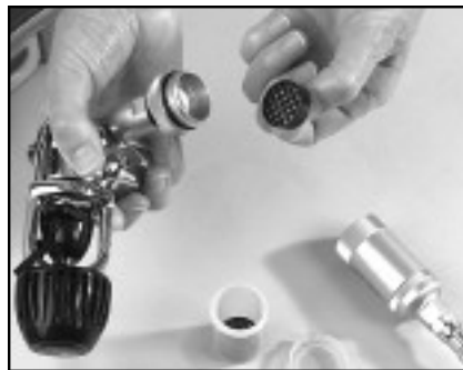
Step 11: Pick up the Activated Charcoal Filter by the tab on its top. Install the Activated Charcoal Filter in the First Stage Body Joint.
