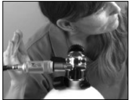
Step 15: Listen for any leakage of air from the Bio-Filter. If you detect any leakage, turn off the tank, purge the regulator, and check the assembly to locate the source of the leak. You can also check for leaks by spraying the Bio-Filter with a mild solution of soapy water.
