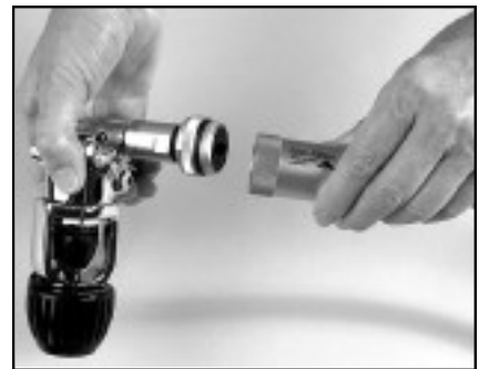
Step 12: Thread the Moisturizer Housing onto the First Stage Body Joint and tighten until snug. Do not use any tools to tighten this connection.
