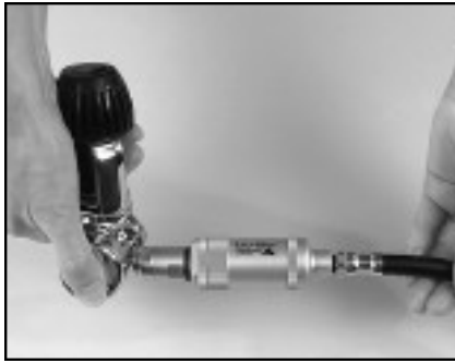
Step 4: Carefully thread the hose into the Moisturizer Cap on the Bio-Filter.
